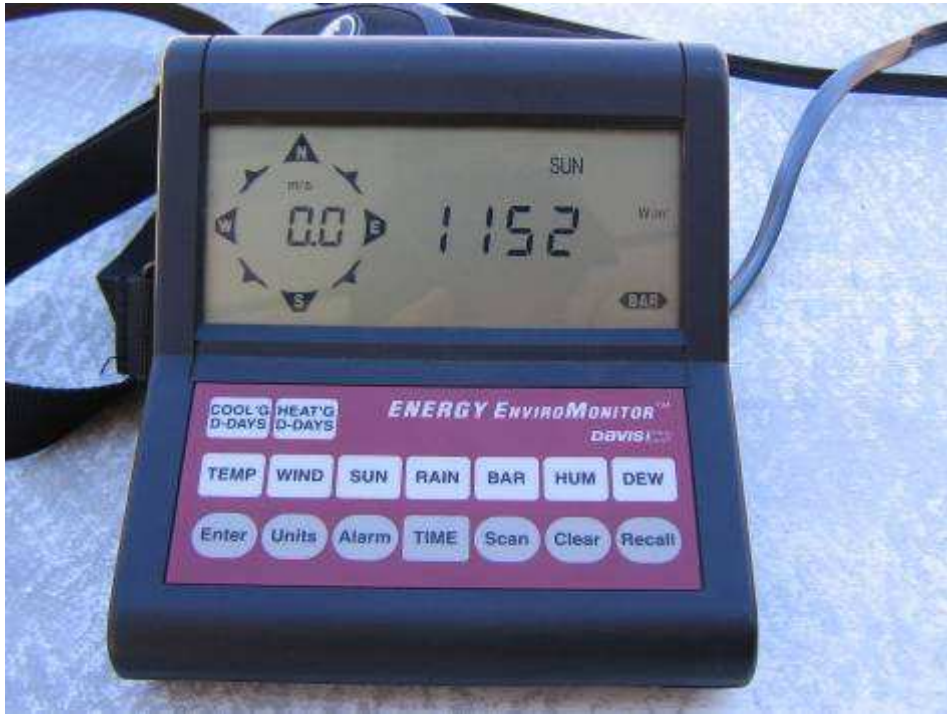
Figure A.3: Solari Meter: Measurement of solar radiation ( 1152 \text{ W/m}^2 ) near guest house.
