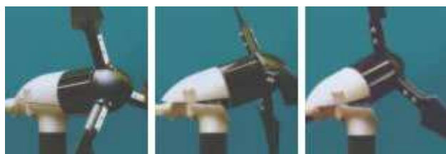
Figure 4: Whisper Wind Turbine during high wind speeds
