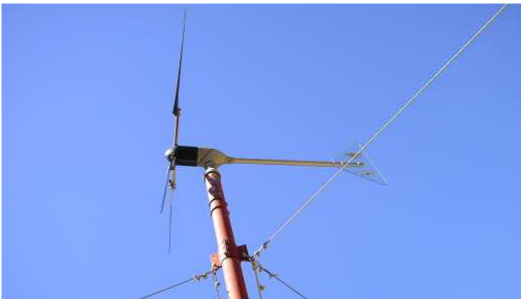
Figure A.6: The Whisper Wind Generator - Model Whisper 200 (1000 W maximum output @ 11.6 m/s wind speeds)
