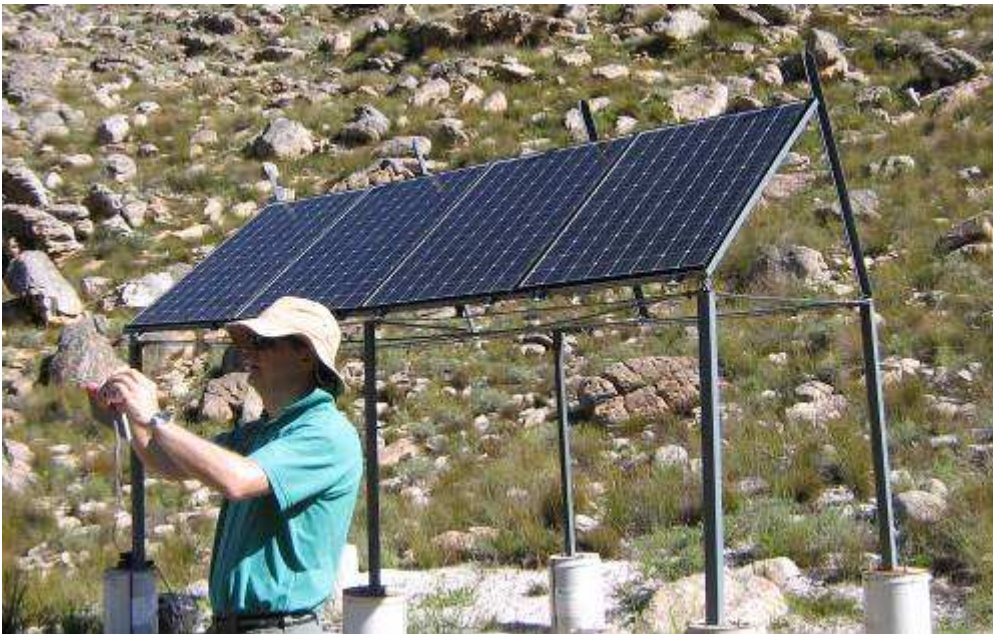
Figure A.3: Solari Meter: Measurement of solar radiation ( 1152 \text{ W/m}^2 ) near guest house.
